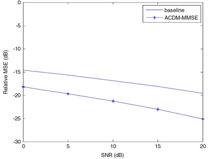
Fig. 3. Relative log mean-squared error of static MFCC features for baseline and proposed front-ends on Test Set C by SNR level.
