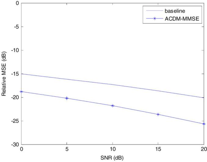
Fig. 1. Relative log mean-squared error of static MFCC features for baseline and proposed front-ends on Test Set A by SNR level.
